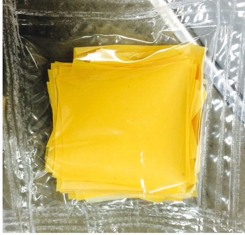
Figure 4.1: The new material candidate, polyimide without glass cloth(PI w/o GC) 5 \mu\text{m} and epoxy 75 \mu\text{m} .
